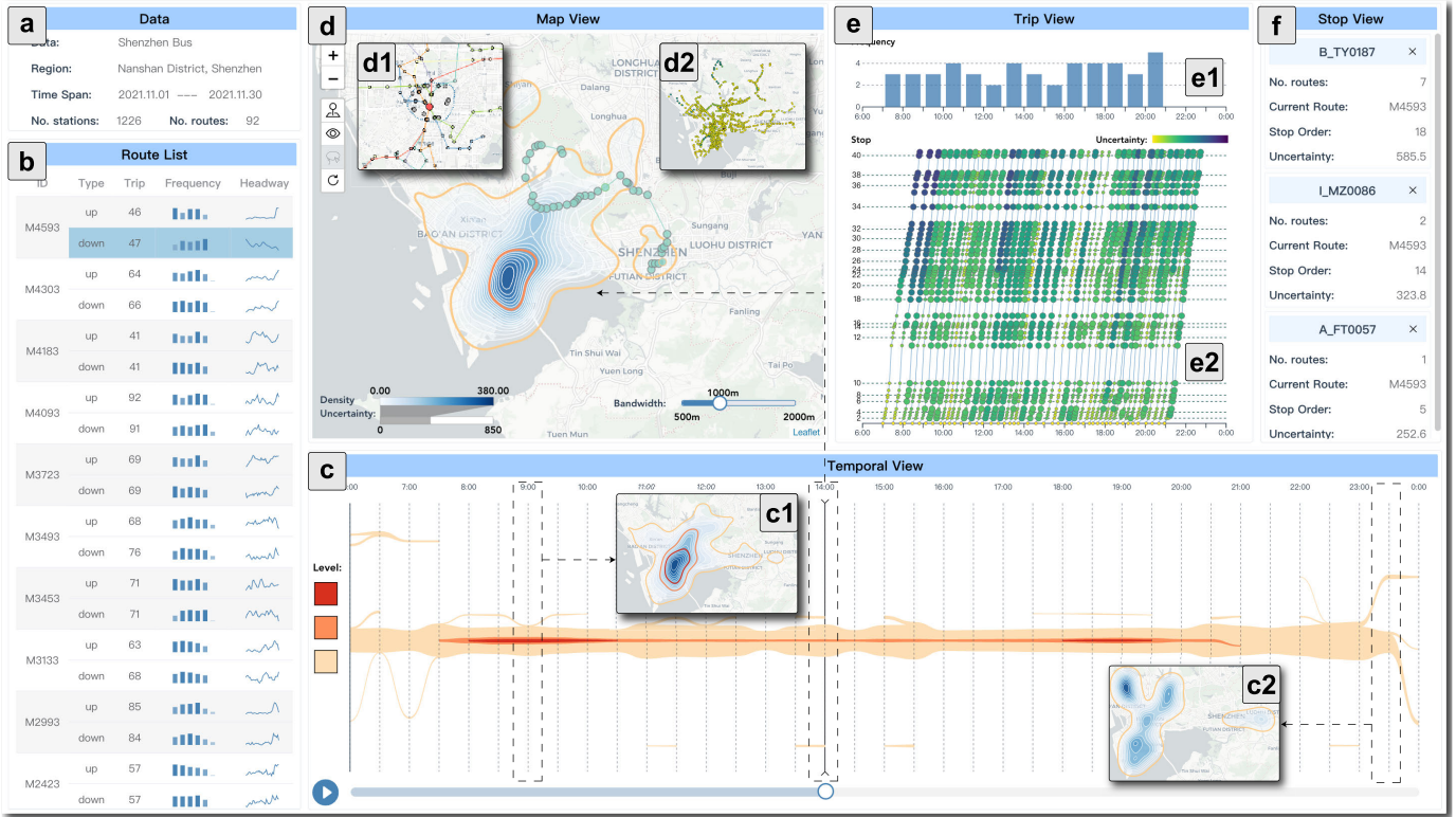
Fig. 7. Interface of MetroBUS system for the input dataset (a). Route List (b) view displays general information of all routes, including route ID, route type, number of daily trips, frequency, and headway. Temporal View (c) provides an overview of and allows users to explore the evolution of uncertainty over time interactively. Map View (d) presents region-level uncertainty distribution over space and user-selected bus route. Trip View (e) displays detailed information of a specific route, including frequency (e1) and trip-level uncertainty information (e2). Stop View (f) displays the finest stop-level uncertainty information of the selected stops.
