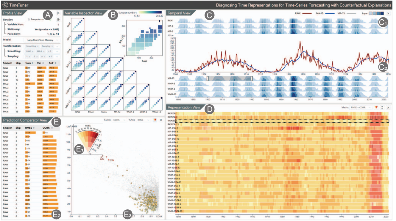
Fig. 4: The interface of TimeTuner . Profile View (A) provides information about the input dataset and an overview of all representations. Variable Inspector View shows the localized distribution of different representations of univariate time series (B), helping users compare different smoothing methods. Temporal View (C) presents global and local information of multiple representations/variables using horizon graphs. Representation View (D) displays different time-series representations for users to explore, which shares the same color coding with Prediction Comparator View (E).
